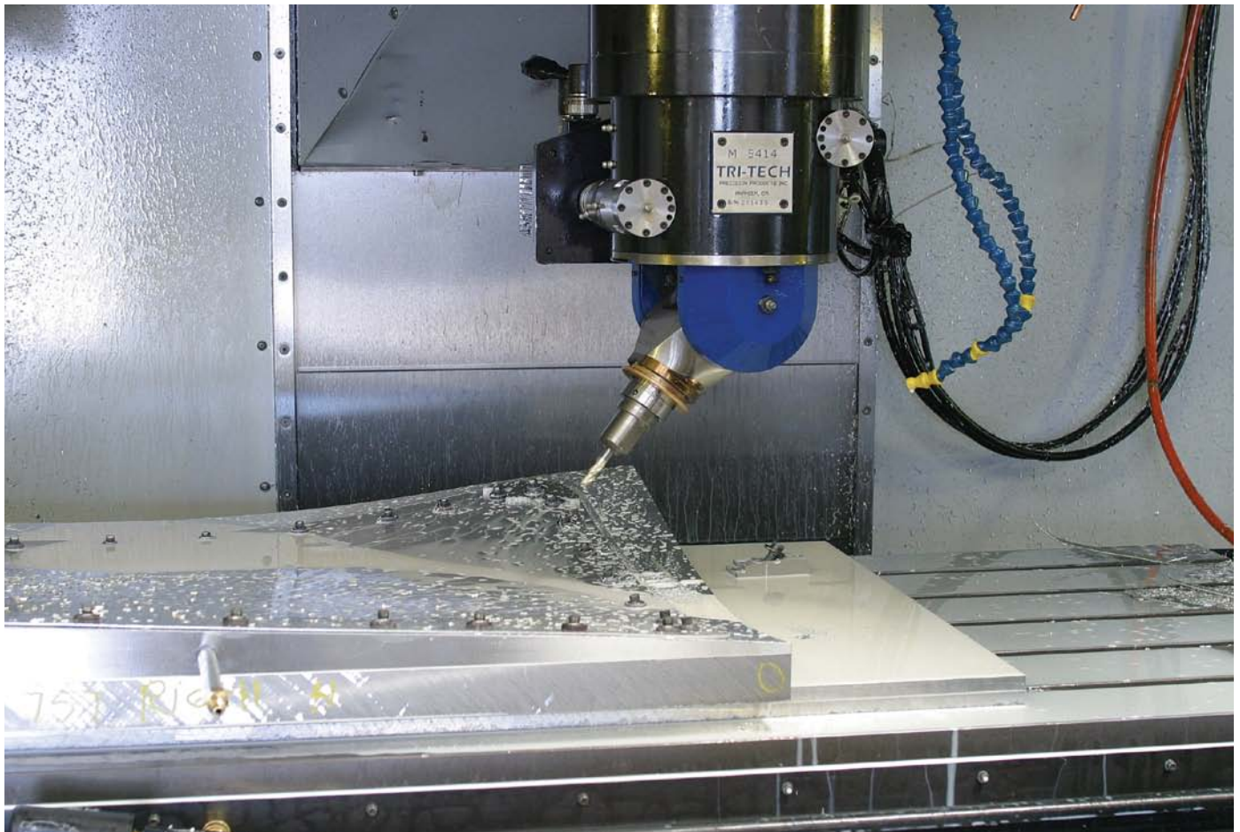
View of the Tri-Tech 5-axis head at work producing a 757 front window frame. The head is lightweight, quick and easy to install, and tilts a full 90° with 360° rotation to allow total control. MY Machine bought the head as a low-budget way to land a major 5-axis contract.
